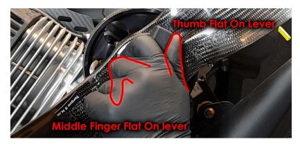
Hold the handle in this position as you loosen the mechanism. Do not let go of the handle or rotate your hand.
