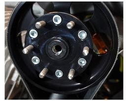
4. Using a torque wrench with a 5mm hex bit, tighten mounting bolts using a standard crisscross pattern to the following specifications:
